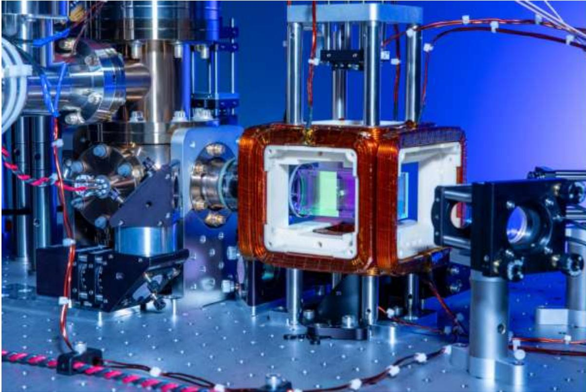
*The Aquila magneto-optical trap in QuEra's facilities*
