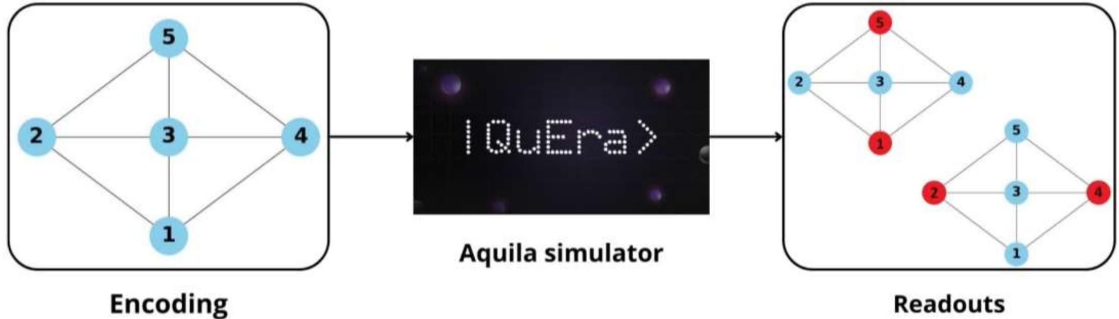
The objective is to use the **Deep Reinforcement Learning** to decide the scheduling for the input pulse parameters for **Aquila neutral atoms quantum computer** in order to maximize the probability to find in the output a configuration that solves the **Maximum Independent Set** problem for an arbitrary graph.
