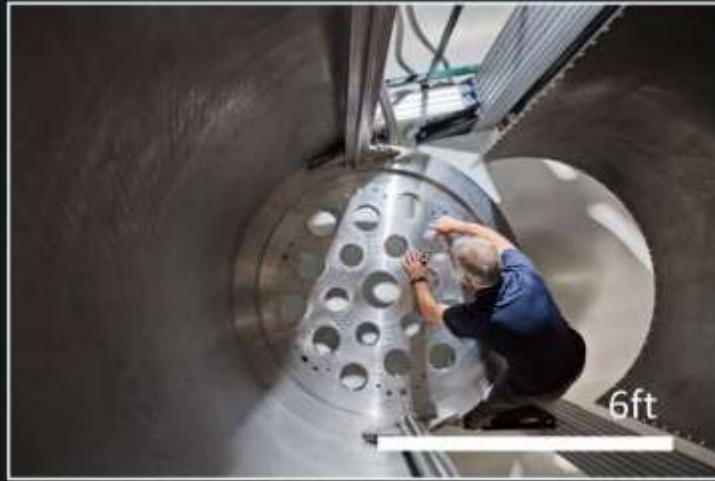
An IBM engineer working on the custom-built dilution refrigerator casing for a single QPU
